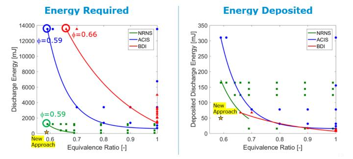
Results showing reducing in energy required for new ignition approach. For comparison, the other data shown include measurements made using repetitive nanosecond pulses driving either (a) a j-gap spark plug geometry (NRNS), (b) a star-point geometry designed by Tenneco (ACIS), or (c) a custom plug with the center electrode encased in dielectric (BDI). Data taken with Isaac Ekoto at Sandia National Laboratories CRF.
