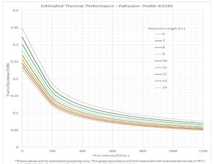
Actual thermal performance relies heavily on many application parameters. Contact Aavid for assistance in determining more accurate thermal performance in your specific application.
