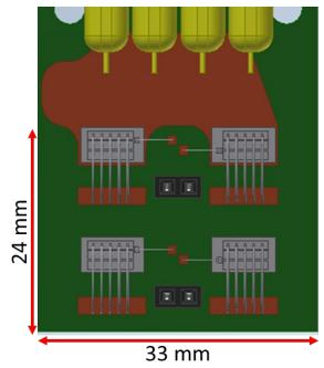
Board with bare die and wire bonds; dimensions give the footprint for this chipon-board approach
