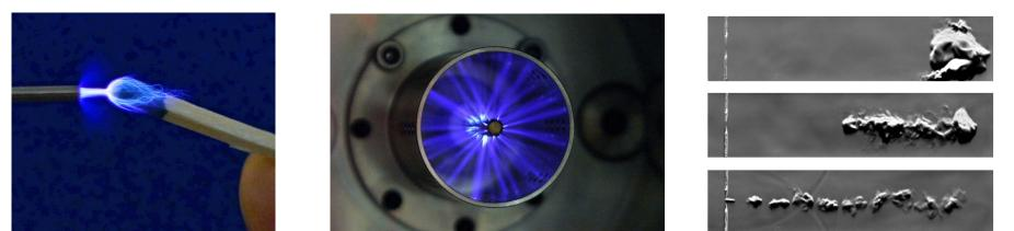
Demonstrated stable operation at: λ>2, EGR>40%, ignition pressure >100 bar
